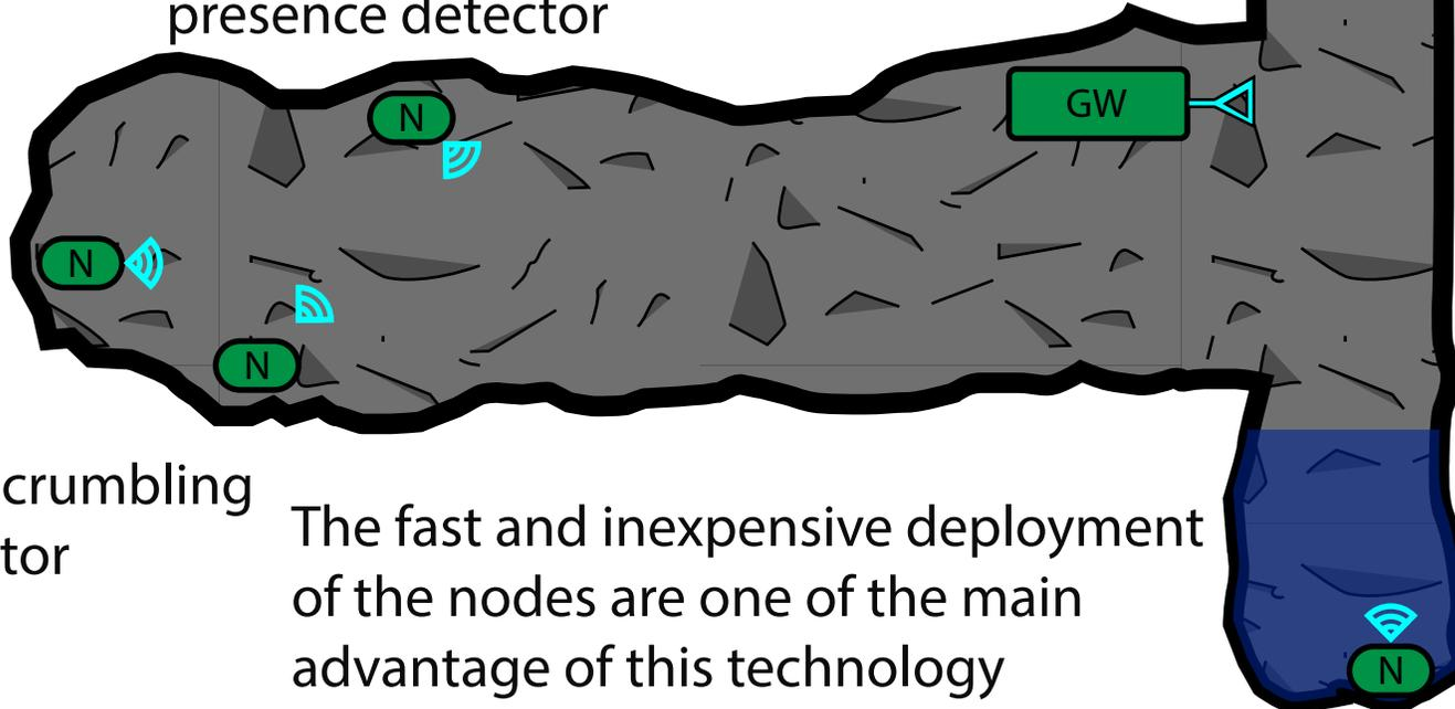
Node3: Movement, crumbling and vibration detector
